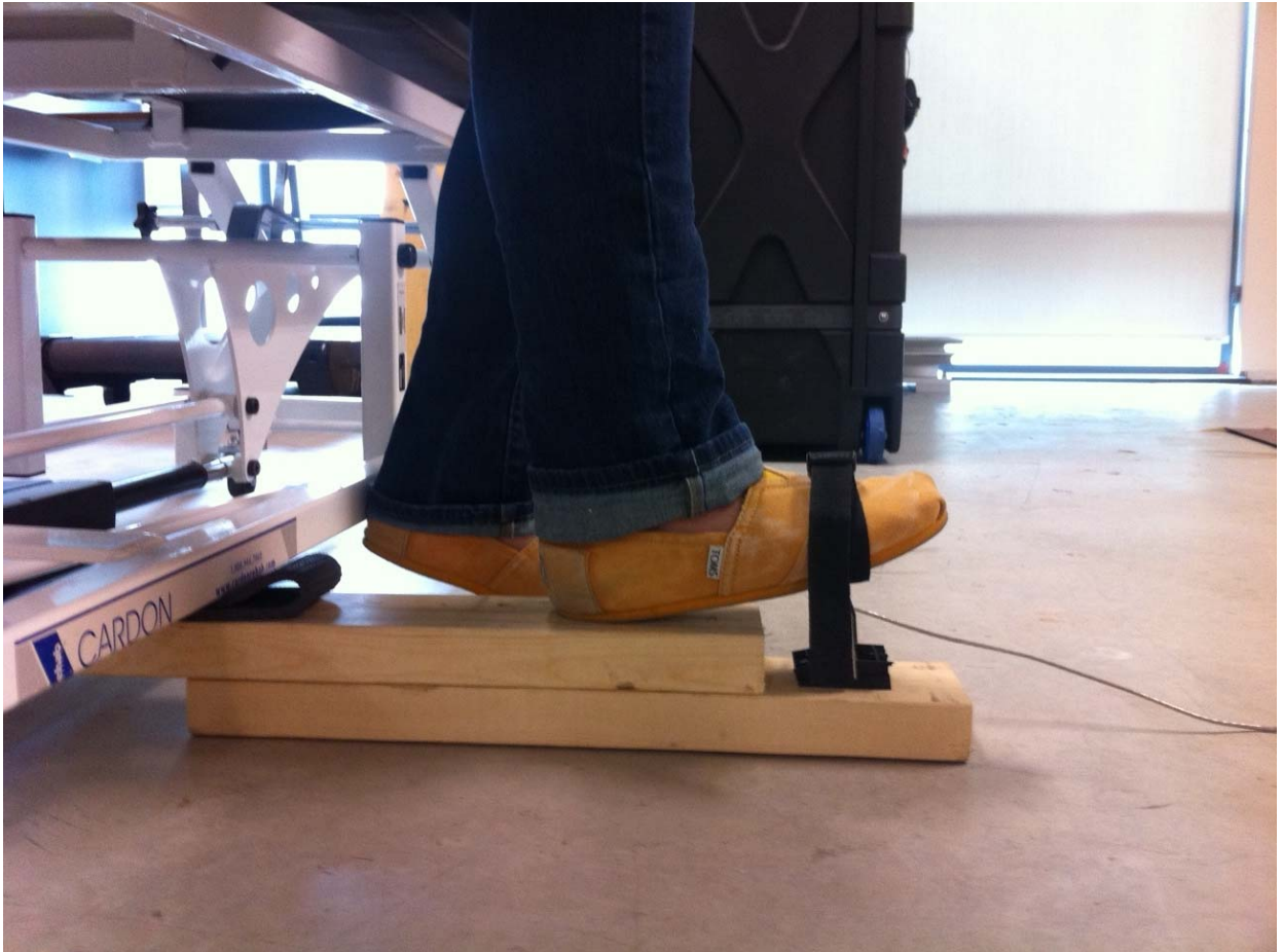
Figure 2.1: Picture of the set up position for testing maximal voluntary isometric contractions of the ankle dorsiflexor and plantarflexor muscles.
